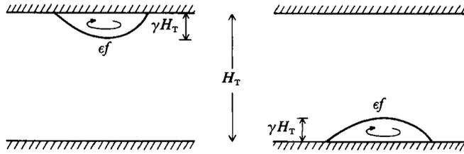
FIGURE 1. Cross-section of the basic state: a vortex is solid-body rotating at an (anticyclonic) angular speed  $-\epsilon f$  ( $0 < \epsilon < 1$ ), and its maximum thickness equals  $\gamma$  times the total depth of the system ( $0 < \gamma < 1$ ).
