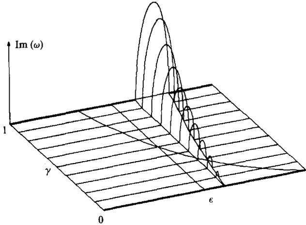
FIGURE 9. As in figure 7, for one Poincaré and one Rossby component  $\mathcal{P}_1^+$  in the vortex layer and  $\mathcal{R}_0$  in the environment layer (Sakai instability);  $|m| = 3$ . The instability region starts at  $\epsilon = \frac{2}{3}^+$ ,  $\gamma = 0^+$ .
