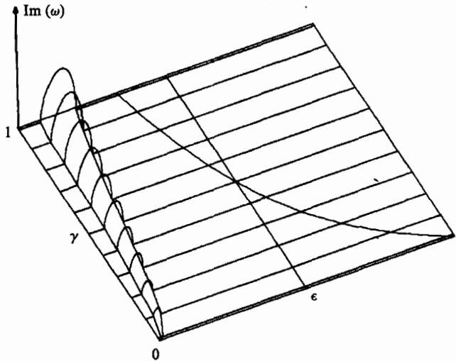
FIGURE 7. Growth rate as a function of  $(\epsilon, \gamma)$ , taking only two Rossby components:  $\mathcal{R}_1$  in the vortex layer and  $\mathcal{R}_0$  in the environment layer (baroclinic instability); the azimuthal wavenumber is equal to three. The boundaries of the regions of figure 2 are also drawn: notice that, for this type of instability, it is  $\text{Im}(\omega) \equiv 0$  where a growing perturbation in the vortex layer was predicted to be Poincaré-like.
