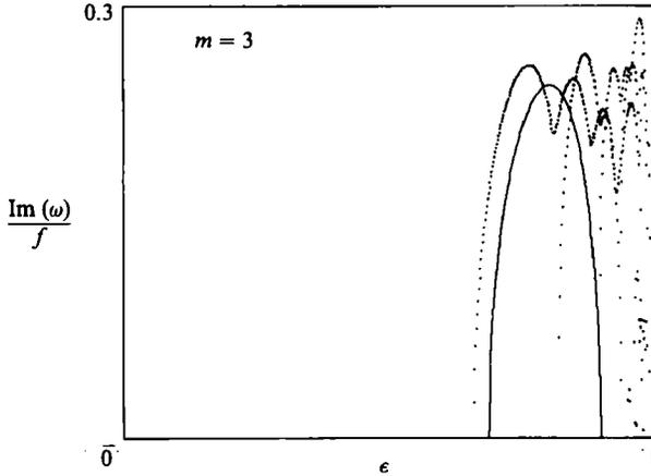
FIGURE 14. As in figure 8, for the case of Kelvin–Helmholtz instability. —, the two components of figure 13, ..., the following twelve Poincaré components:  $\mathcal{H}^+$ ,  $\mathcal{P}_1^+ \dots \mathcal{P}_5^+$  in the vortex layer and  $\mathcal{P}_0^- \dots \mathcal{P}_5^-$  in the environment layer.  $\gamma = 0.9$ .
