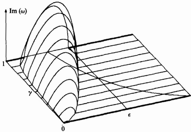
FIGURE 11. As in figure 7, for the hybrid component  $\mathcal{H}^+$  in the vortex layer and the Rossby component  $\mathcal{R}_0$  in the environment layer: this hybrid instability goes continuously from baroclinic instability (as in figures 7 and 8) at low Rossby numbers  $\epsilon$ , to Sakai instability (as in figures 9 and 10) at larger values of  $\epsilon$ .
